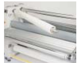
Swing-out Shaft for easy loading of materials
